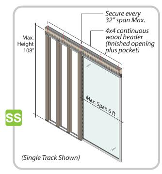
2 Surface Mount - Single or Double Track Pocket: Up to 144" W Panel Coverage x 108" H requires continuous 4x8 wood header
