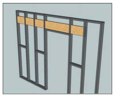
When mounting a barn door, there must be structure in the walls to support a minimum of 300 lbs throughout the entire track length. A continuous structural wood header (4x8 minimum) is required (see structural requirements section for more information).
