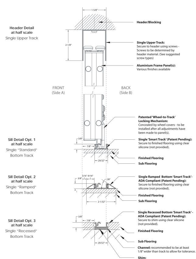
Shim height to be determined by finished floor height. Track CANNOT be recessed more than 3/8" into the flooring
